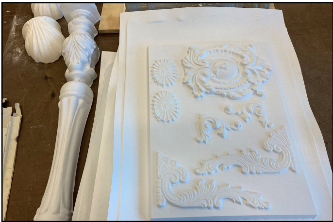
To the right are some formed plastic sheets from bucks the students prepared. These can now be applied to scenery and props to recreate durable and lightweight architectural ornamentation.
